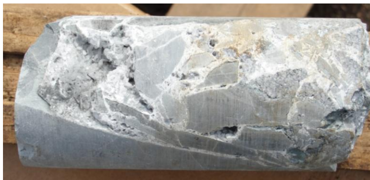
Figure 9. Brecciated fracture zone with secondary calcite deposit from a depth of 64.92m in TG4.
