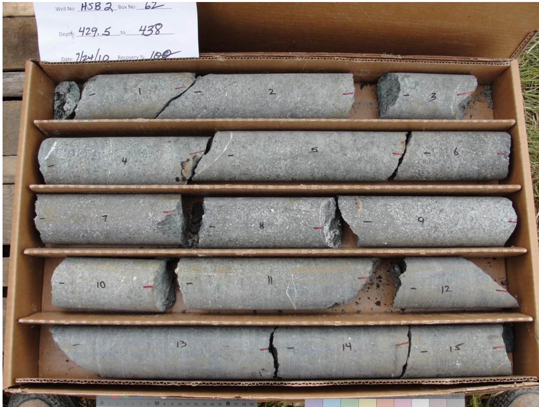
Figure 6. Example of a typical 3.05m core box from well TG2 containing andesite (sections #1-11 in photo) and andesitic tuff (sections #11-15 in photo).
