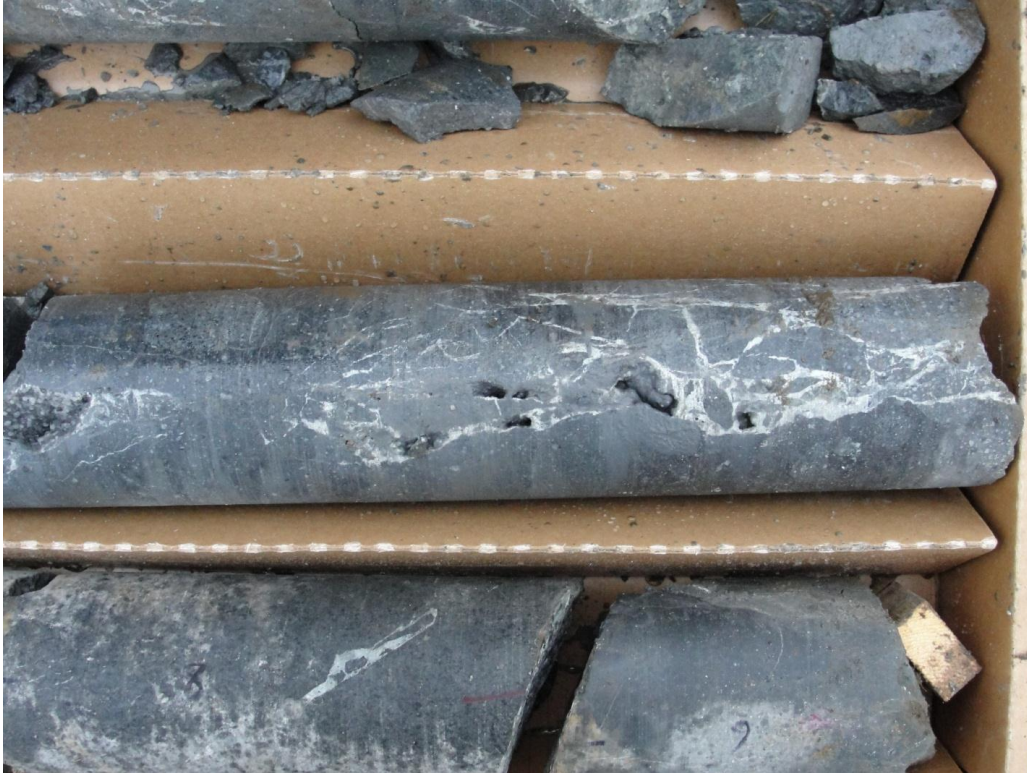
Fig 8. Fractured zone from 56.39m-56.7m in well TG4. Fractures are filled with amorphous calcite, epidote, and sulfides (pyrite, arsenopyrite, and possibly cinnabar).
