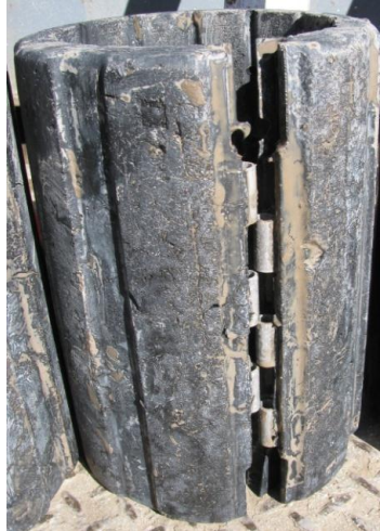
Figure 5. NRP sleeve after the initial field test, which included drilling 910 m in 130 rotating hours. Although scratched by the formation abrasion, there was no significant wear or damage to the sleeve.
