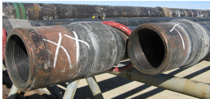
Figure 6. Bonded material shown on the box ends of two joints of drill pipe.
