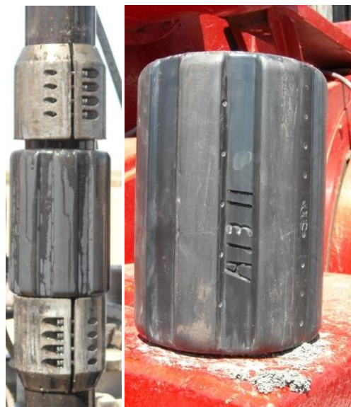
Figure 8. NRP assembly and sleeve run 615 m into open-hole during the cleanout run.
